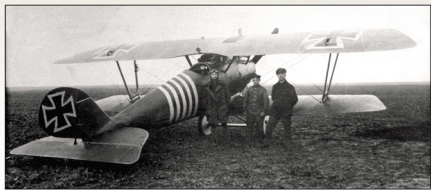
Max Hitschler's Jasta 18 Pfalz D.IIIa. In keeping with contemporary German fighter design practices the Pfalz D.III/IIIa upper wing was constructed as a single part but, unlike the Albatros D.III and D.V, the Pfalz centre section (which contained the radiator and a fully enclosed gravity fuel tank) was skinned in plywood before being covered with linen. Note the rear view mirror (E39), anemometer (E41) mounted to the front left strut and the irregular white border of the right upper wing cross as it meets the aileron, indicating a possible replacement.
