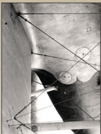
Wing rigging detail from Palz DIII 1405/17 which is identical to those of the DIIIa
