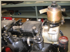
Large air pump (E28) characteristic of the 180ps Daimler Mercedes D.111A.
