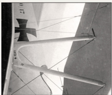
Wing rigging detail from Palz DIIIa 6050/17.
