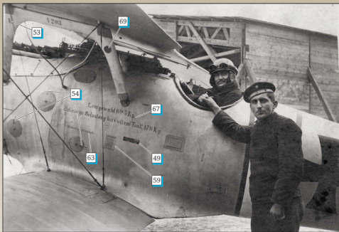
Pfalz D.IIIa 4208/17 of Marine Field Jasta (MFJ) 1 showing the initial style of weight table [67]. The blunt ends of the cabane struts have been painted after being attached to the struts. Note the worn appearance of the silver grey paint and the staining under the fuel lines from the gravity tank. (Greg VanWyngarden)
