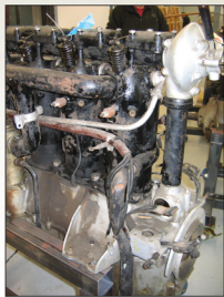
Rear left view showing the empty magneto mounts, water pipe and spark plug details.
